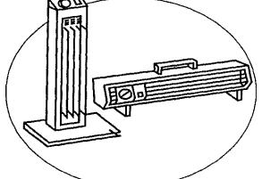
Place heater level and on the floor so it won't tip over. Make sure no nearby items can fall onto the heater and ignite.
